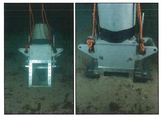
Figure 2.2: Diver operated Sediment Profile Imaging camera. The left-hand image gives a view of the camera at the sediment surface. The right-and image shows the SPI camera when inserted into the sediment
